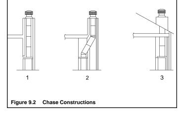
**WARNING!** You must install false ceilings and ceiling firestops at each floor of the chase or every 10 ft (3.05 m) to control spread of fire.
